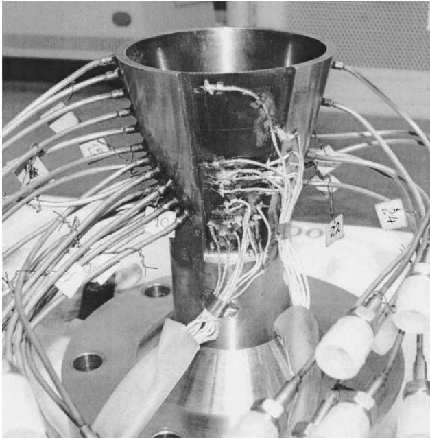
Fig. 12 Temperature sensors mounted to nozzle model for hot-gas tests.
